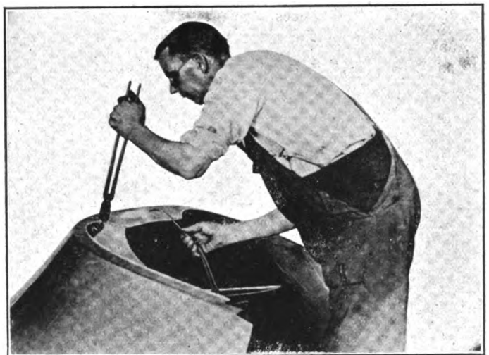
Fig. 2—Welding in front panels of cowl and method of holding sheets
